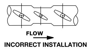
Combination with all valve stems in the same direction accelerates possible noise, vibration, & erosion problems.
