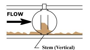
INCORRECT INSTALLATION Sludge builds up on disc
