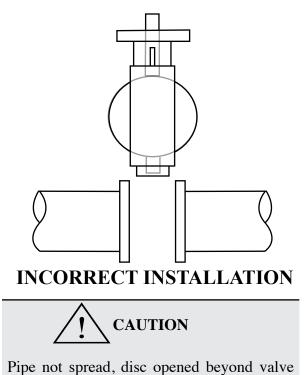
Figure 1 – Insert Resilient Seated Butterfly Valve Between Flanges
