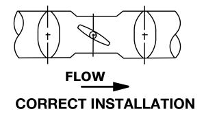
Combination with the stem of the control valve at right angle to those of other valves tends to cancel the drift of the fluid, and reduces noises, vibration, and erosion.
