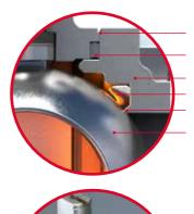
Metal-to-Metal Contact Body Seal Valve Body Burned Seat Secondary Metal Seat Ball
