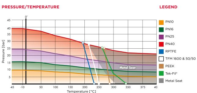
Note: Carbon steel valves limited to -29°C.
