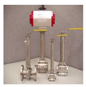
The production, transportation and storage of liquefied gases present several technical problems to valve designs. The integrity of the stem seals at very low temperatures is the major hurdle that must be overcome. Specially designed valve extended bonnets installed to valves offers a safe and efficient method to accomplish stem seal integrity.
