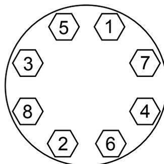
**Figure 3 – Initial Centering & Flanging of Valve**
