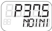
The “P-manual mode” is preset for the positioner in the as-delivered condition. The digital display of the positioner shows the current potentiometer position in the upper line. “NOINI” blinks in the second line of the digital display. You can move the actuator using the decrement and increment buttons. Switch to “Configuration” and “Initialization mode” to adapt the actuator as per the positioner.
