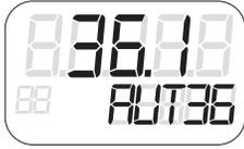
Automatic is the standard mode. In this mode, the positioner compares the setpoint position with the actual position. The positioner moves the actuator until the control deviation reaches the configurable dead zone. A fault message is displayed if the dead zone cannot be reached.
