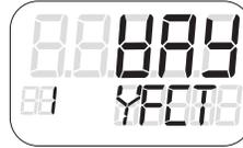
To get to the “Configuration” mode, press the operating mode button for at least 5 seconds. You can use the “Configuration” mode to adjust the positioner individually as per your actuator and start commissioning or initialization. The positioner reports the “Configuration” mode with a configurable fault message. A position feedback or display of limits A1 and A2 is not possible.
