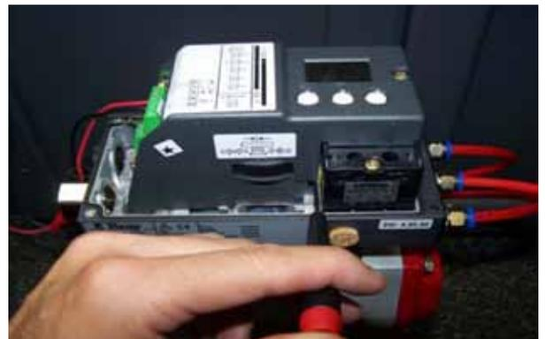
**Step 8:** Adjust the yellow wheel underneath the terminals using a 4 mm wide screwdriver to the neutral position (Midway between 33° and 90°)
