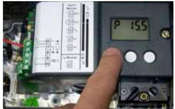
**Step 3:** Once the configuration mode has been initialized, parameter 1 is displayed on the positioner window. Parameter 1 allows the user to select the type of actuator being used with the device.
