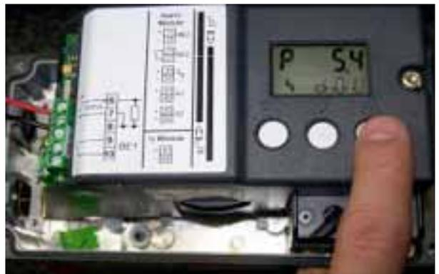
**Step 8:** Upon completion of a successful calibration, the status line will display "FINSH".
