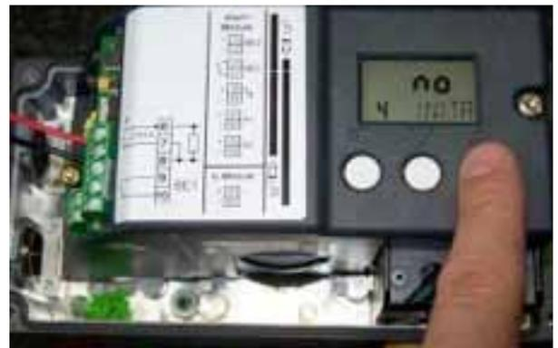
**Note:** *If the error shown is displayed on your positioner during Run 1, the lower tolerance (down tolerance) of the adjustment wheel has been exceeded. (If you don't see any error during calibration, proceed to step 8, otherwise continue reading)*
