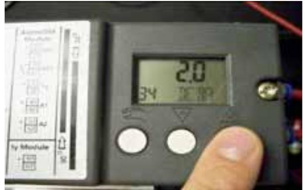
**Step 18:** Scroll to the 'Tight Closing with Manipulated Variable' parameter – YCLS, #39 and select 'uP do' by pressing the '+' button.
