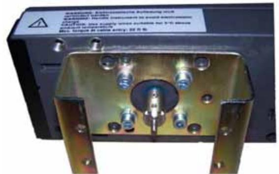
**Step 4:** Place the indicator on the base of the coupler.
