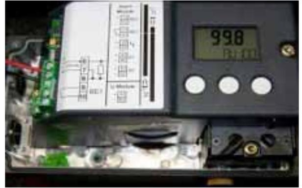
**Step 14:** Upon completion of calibration, insert an ordinary 4mm wide screwdriver into a slot located under the adjustment wheel, and move the wheel to the left until you can feel that it clicks in. This helps prevent the clutch wheel from slipping during actuation.
