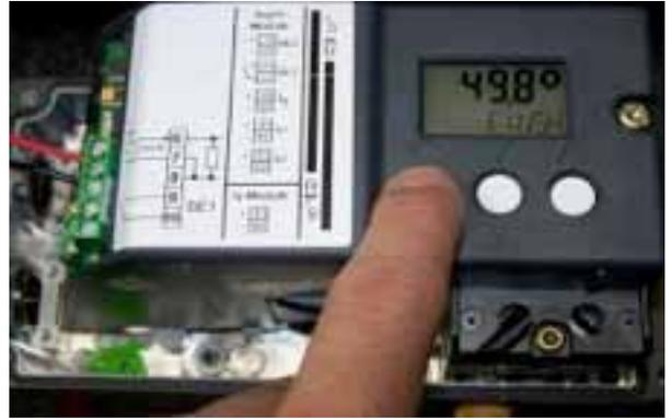
**Step 10:** The device will now be in 'MANUAL' mode. The display should resemble the above screen.
