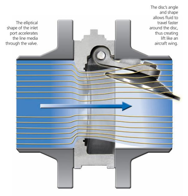
**CHECK RITE SEATS** Zero leakage shut off, even at 0 psi, is achieved through lapped metal seating surfaces. The seat and the disc edges are precisely machined then hand polished for a perfect fit. The disc hinge provides an even force at the disc to seat contact point, ensuring a uniform seal. Controlled tolerances maintain the proper disc to seat alignment. The spring assisted closure tension holds the disc in place when line pressure is removed.
