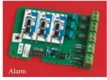
**Programmable Electronic Switches** (Alarm) Two semiconductor switch outputs and one alarm output may be programmed to activate at various travel positions. One digital input is also included.
